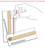
**Step 6:** Move the arm by pulling on the rubber bands. Pulling on one rubber band makes the arm bend, while pulling on the other makes the arm straighten.
